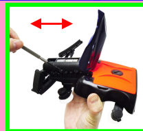
Release the cover screws 解開雨刷器蓋的螺絲
